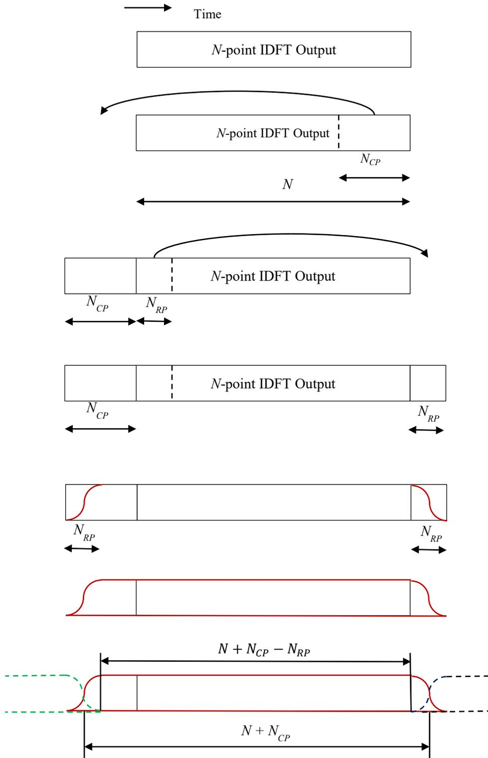
**Figure 17 - Cyclic Prefix and Windowing Algorithm**
