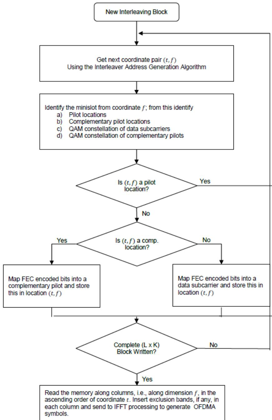
**Figure 11 - Interleaving a Grant within an OFDMA Frame**
