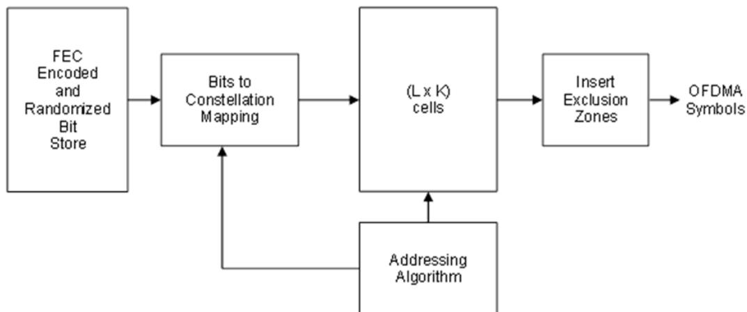
**Figure 10 - Sample Interleaver Block Diagram**
