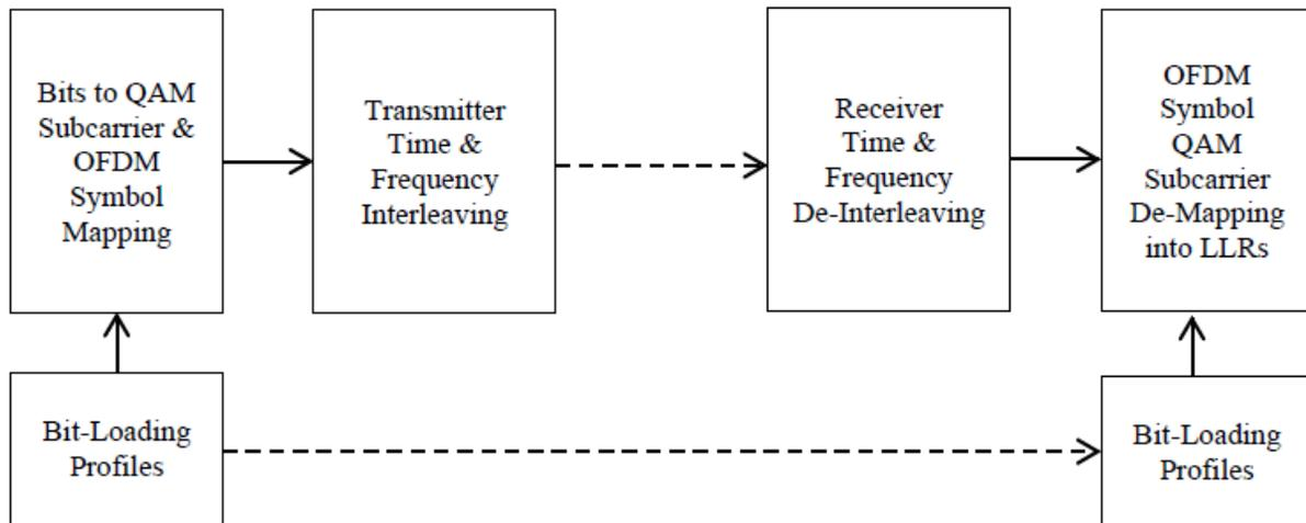
**Figure 53 - Bit Loading, Symbol Mapping, and Interleaving**
