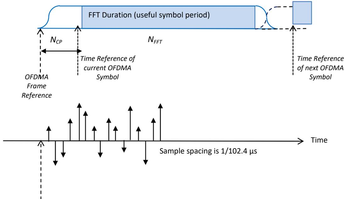
Figure 19 - Time References for OFDMA Symbol and Frame
