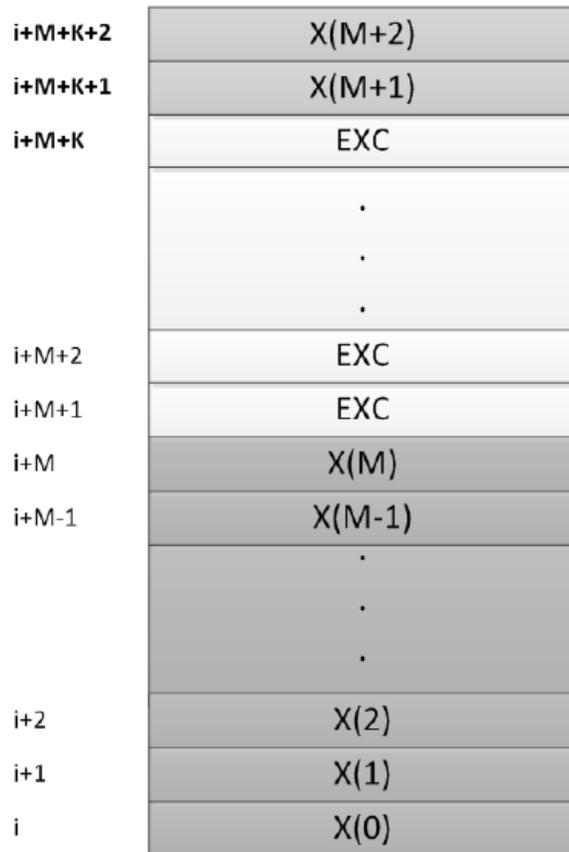
**Figure 28 - Initial Ranging Preamble and an Exclusion Band**
