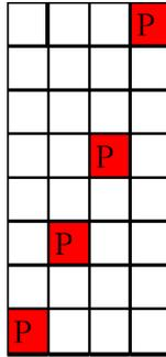
Figure 43 - Pilot Pattern for Subslots with 8 Subcarriers
