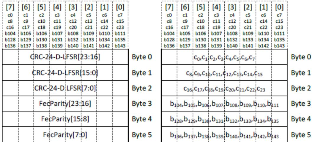
Figure 75 - Mapping FEC Encoded CRC-NCP Bytes into a Bitstream
