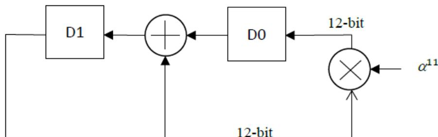
Figure 52 - Linear Feedback Shift Register for Randomization Sequence
