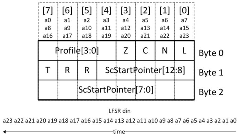
Figure 74 - Mapping NCP Data into the CRC-24-D Encoder
