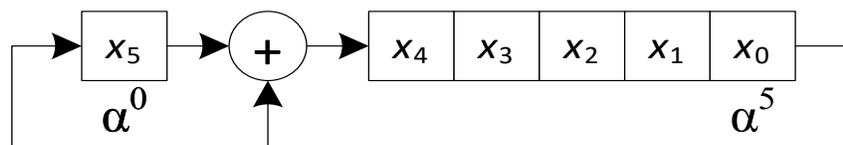
**Figure 57 - Linear Feedback Shift Register**
