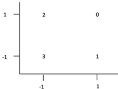
Figure 100 - QPSK Constellation Mapping of  $\{y_0 \ y_1\}$
