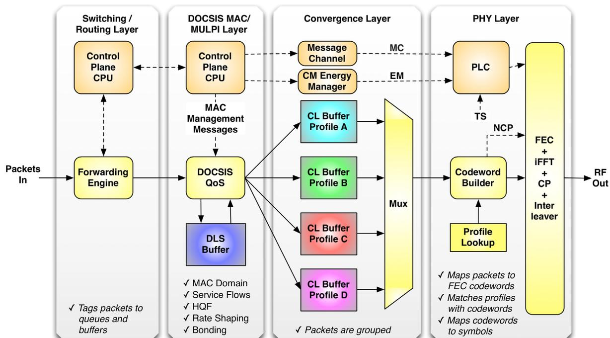
**Figure 89 - Downstream Convergence Layer Block Diagram**
