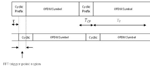
**Figure 16 - Signal with Micro-Reflection at the Receiver**
