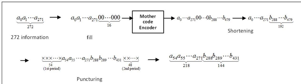
**Figure 32 - Shortening and Puncturing Encoder for the Fine Ranging FEC**
