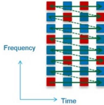
**Figure 87 - Data Mapping for a 4x8 Subslot**
