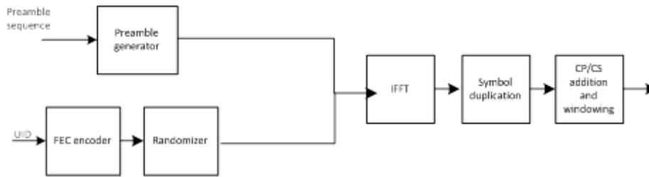
**Figure 31 - Fine Ranging Transmitter Processing**
