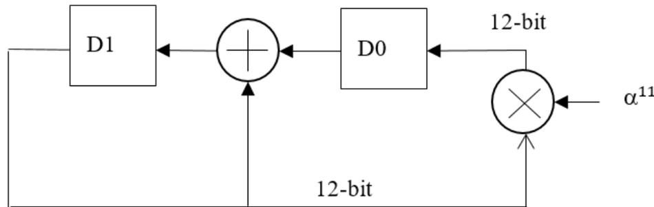
**Figure 68 - Linear Feedback Shift Register for PLC Randomization**
