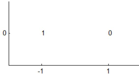
Figure 99 - BPSK Constellation Mapping of  $\{y_0\}$
