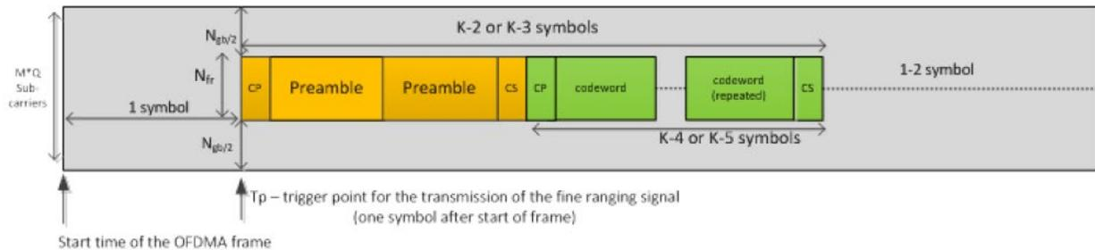
**Figure 30 - Fine Ranging Signal Transmission**
