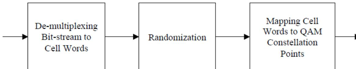
**Figure 50 - Bits to QAM Constellation Mapping**
