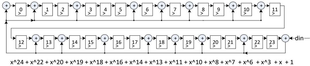
Figure 73 - Polynomial Sequence for CRC-24-D Encoding
