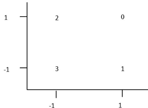
**Figure 79 - QPSK Constellation Mapping of  $\{y(i,0)y(i,1)\}$**
