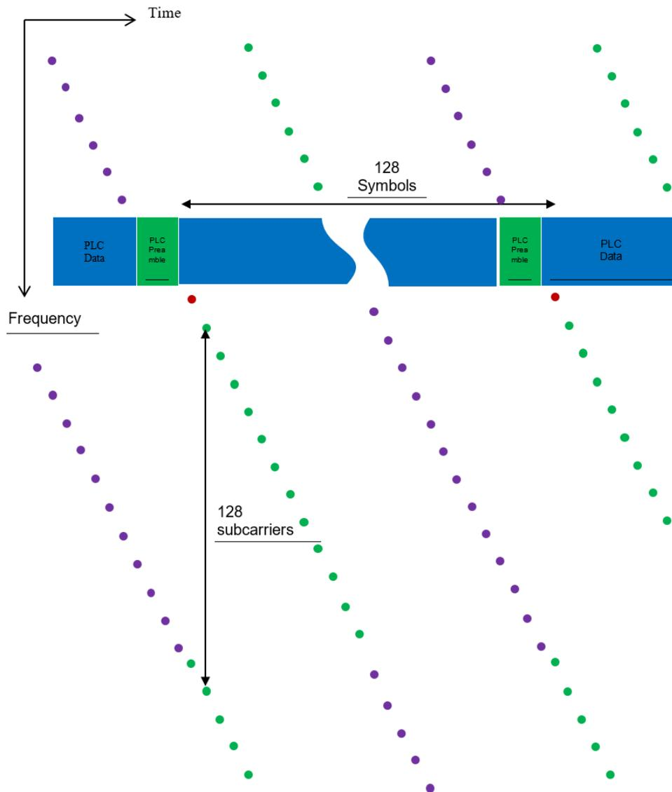
**Figure 82 - 8K FFT Downstream Scattered Pilot Pattern**
