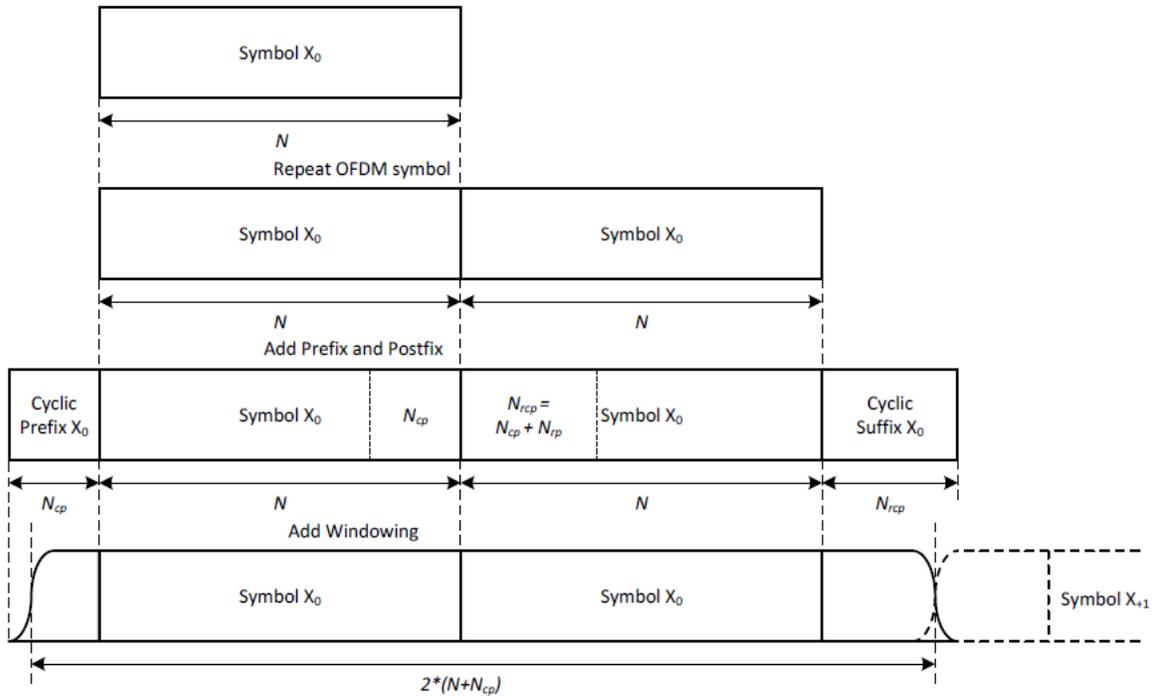
**Figure 26 - Initial Ranging Symbol Pair Structure**
