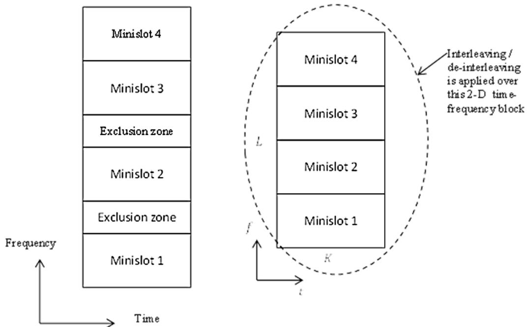
**Figure 9 - Illustrating Minislots of a Grant over which Interleaving is Performed**
