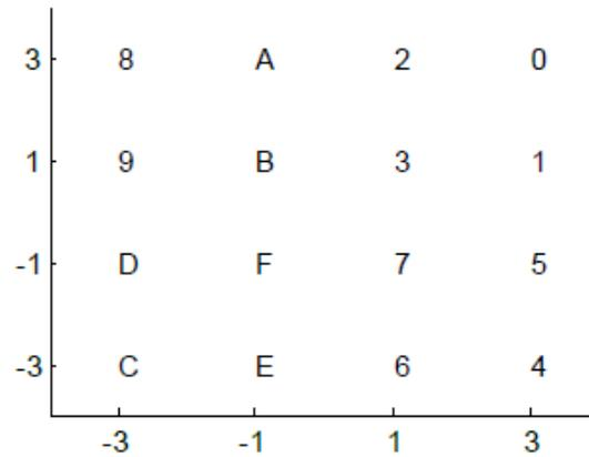
**Figure 78 - 16 QAM Constellation Mapping of  $\{y(i,0)y(i,1)y(i,2)y(i,3)\}$**
