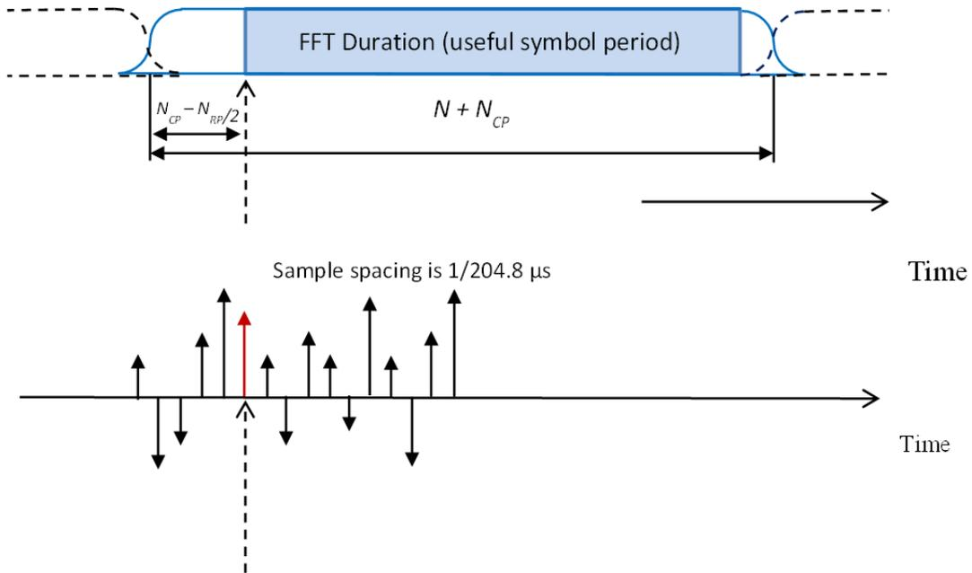
**Figure 70 - Time Domain Representation of PLC Timestamp Synchronization**
