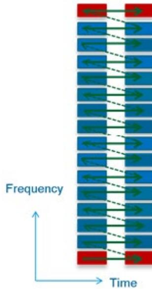
**Figure 88 - Data Mapping for a 2x16 Subslot**
