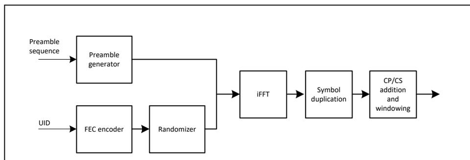
**Figure 24 - Block Diagram of Initial Ranging Transmitter Processing**
