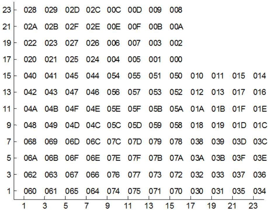
**Figure 109 - 512-QAM Constellation Mapping of  $\{y_2 y_3 y_4 y_5 y_6 y_7 y_8\}$  on to Quadrant 1**
