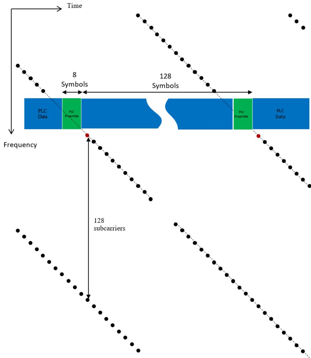
**Figure 80 - 4K FFT Downstream Pilot Pattern**
