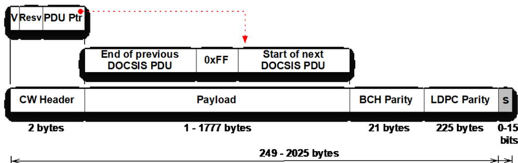
Figure 90 - DOCSIS Frame to Codeword Mapping
