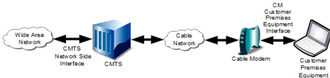
Figure 2 - Transparent IP Traffic through the Data-Over-Cable System
