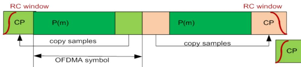
**Figure 23 - Initial Ranging Admission Slot Structure**
