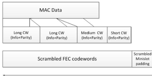
**Figure 6 - Upstream Framing Block Diagram**
