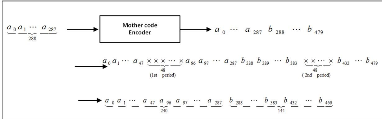
**Figure 64 - Puncturing Encoder for the PLC FEC**
