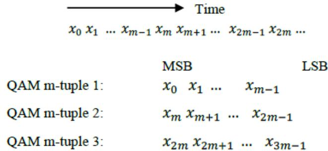
**Figure 13 - Bitstream to QAM M-Tuple Mapping**
