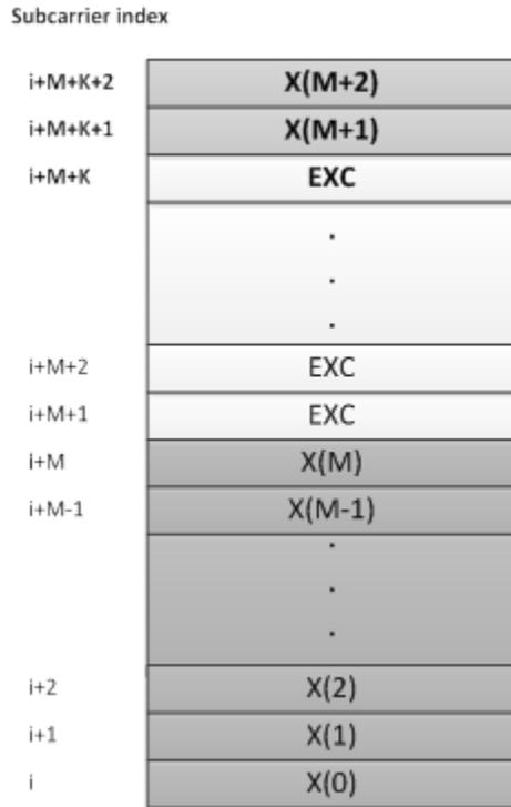
**Figure 34 - Fine Ranging Preamble and an Exclusion Band**
