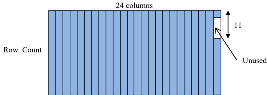
Figure 48 - Bit De-interleaver Block for a Shortened Codeword
