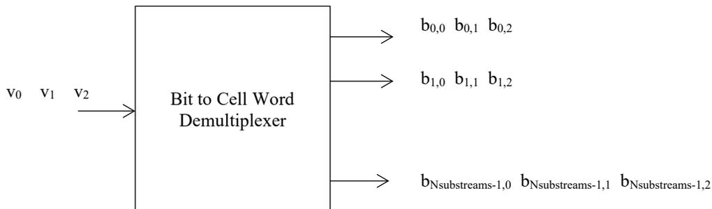
**Figure 51 - Bit-to-Cell Word Demultiplexer**
