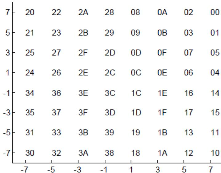
**Figure 77 - 64-QAM Constellation Mapping of  $\{y(i,0)y(i,1)y(i,2)y(i,3)y(i,4)y(i,5)\}$ ...**
