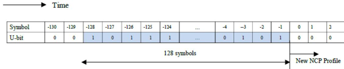
**Figure 93 - NCP Profile Update Bit Setting Immediately Preceding an NCP Bit Loading Profile Change**
