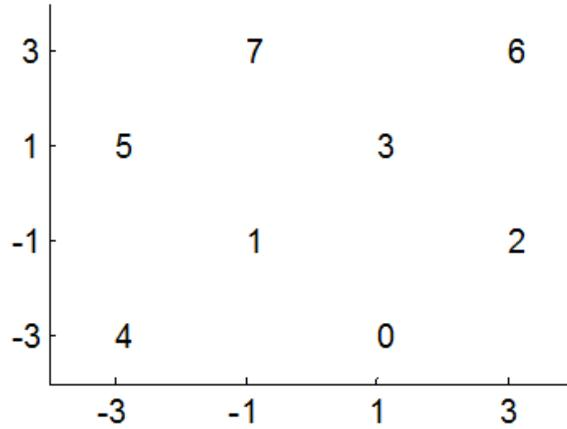
Figure 101 - 8-QAM Constellation Mapping of  $\{y_0 y_1 y_2\}$
