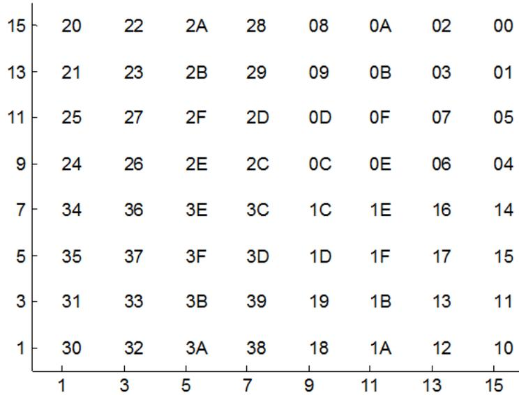
**Figure 108 - 256-QAM Constellation Mapping of  $\{y_2 y_3 y_4 y_5 y_6 y_7\}$  on to Quadrant 1**
