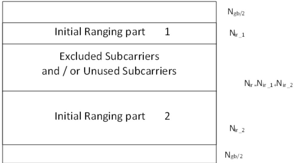
**Figure 27 - Initial Ranging with Exclusions and Unused Subcarriers**
