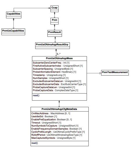
Figure 99 - PnmUsOfdmaAqpTestResultGrp Class Diagram
