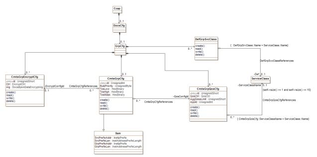
Figure 30 - DOCSIS Multicast QoS Configuration Information Model
