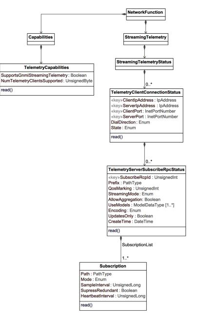
Figure 90 - gNMI Streaming Telemetry Status Information Model
