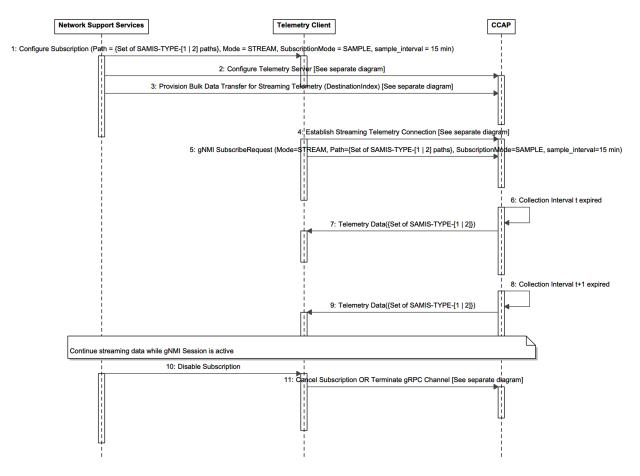
Figure 125 - gNMI Streaming Subscriber Usage Statistics Sequence Diagram
