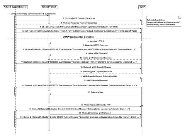
Figure 121 - Dial Out Streaming Telemetry Sequence Diagram
