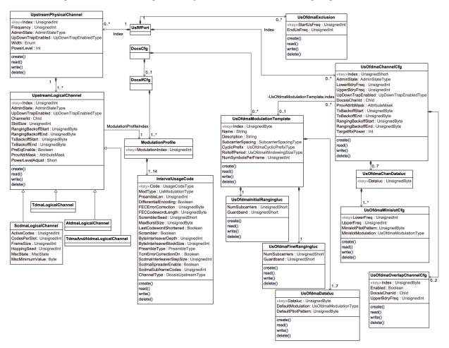
Figure 33 - DOCSIS Upstream Interface Configuration Information Model
