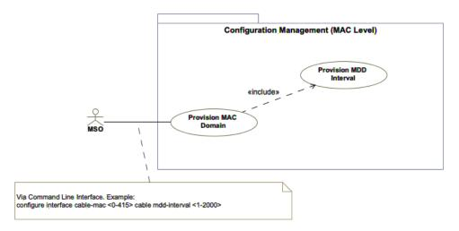
Figure 12 - MAC Domain-Level Configuration Use Case
