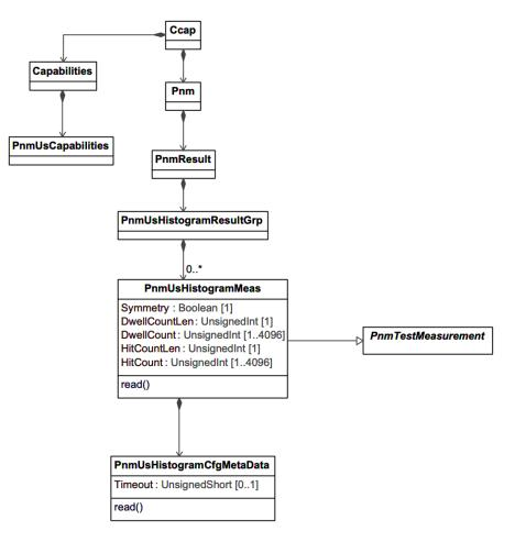
Figure 105 - PnmUsHistogramResultGrp Class Diagram
