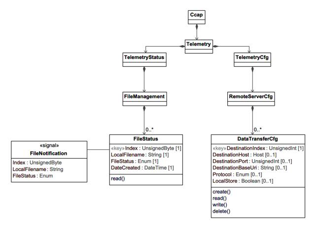
Figure 49 - Bulk File Transfer Class Diagram
