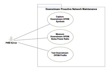
Figure 15 - Downstream Proactive Network Maintenance Use Cases
