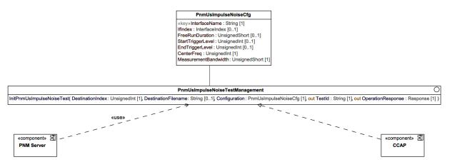
Figure 108 - PnmUsImpulseNoiseTestManagement Component Diagram
