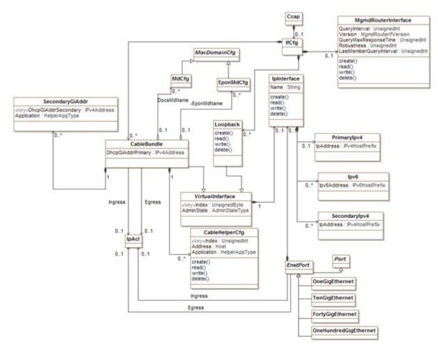
Figure 39 - Interface Configuration Information Model
