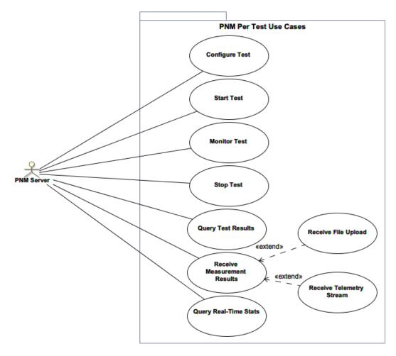
Figure 17 - Common Proactive Network Maintenance Test Use Cases
