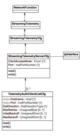
Figure 45 - Streaming Telemetry Configuration Information Model
