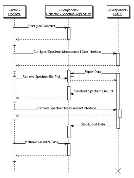
Figure 113 - Sequence Diagram for Streaming of Spectrum Analysis Measurement Data
