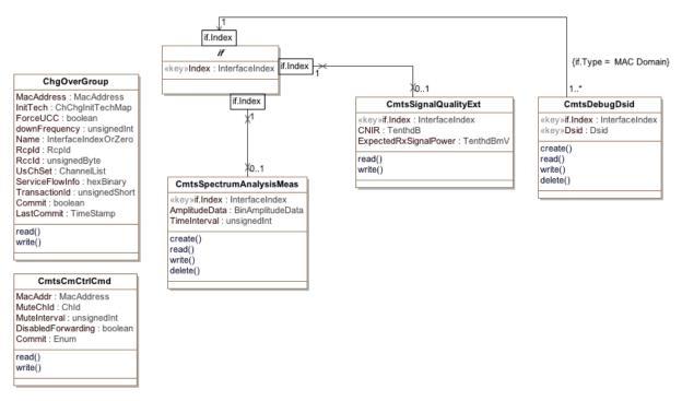
Figure 47 - Performance Management Control and Monitoring Information Model
