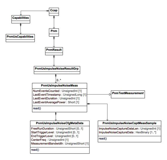
Figure 107 - PnmUsImpulseNoiseResultGrp Class Diagram
