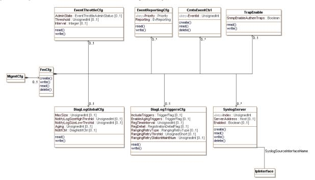
Figure 41 - Fault Management Configuration Information Model
