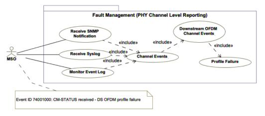
Figure 8 - Downstream Channel Fault Monitoring Use Case
