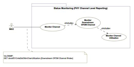
Figure 14 - Downstream Channel Status Monitoring Use Case
