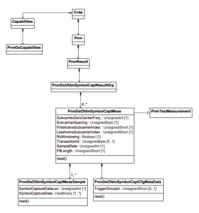
Figure 95 - PnmDsOfdmSymbolCaptResultGrp Class Diagram
