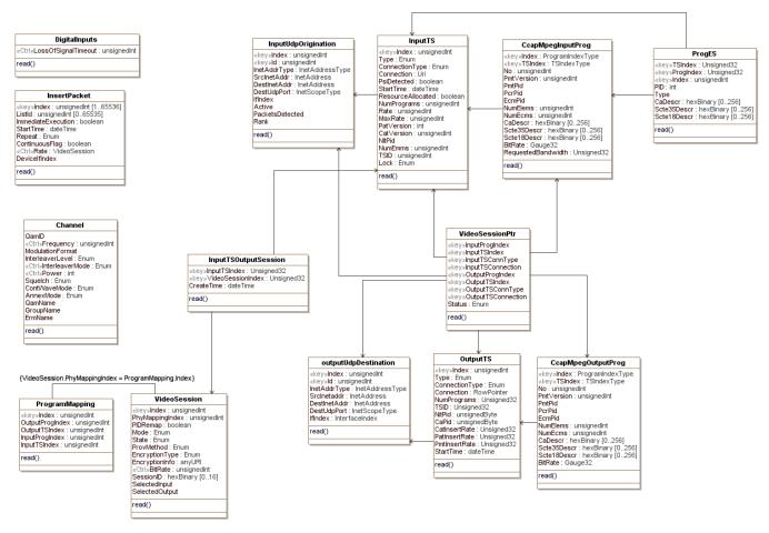
Figure 62 - SCTE-HMS-MPEG-MIB Performance Management State Information Model
