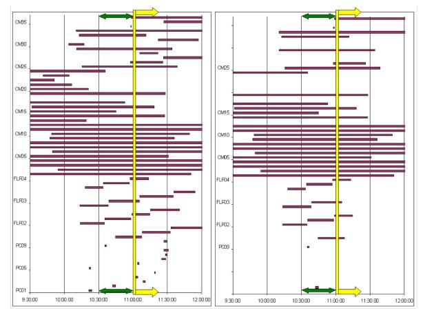
Figure 112 - Set of CM Services in an Arbitrary Period of Time (Left Graphic)Set of Records Associated to the Collection Interval 10:30 to 11:00 AM (Right Graphic)
