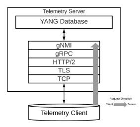
Figure 87 - Streaming Telemetry Dial-in Protocol Stack
