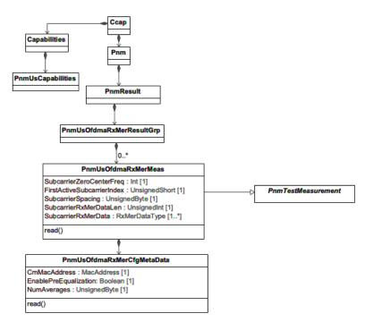
Figure 97 - PnmUsOfdmaRxMerResultGrp Class Diagram
