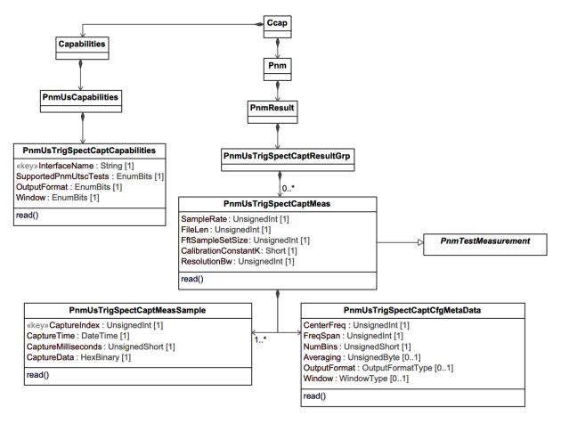
Figure 103 - CCAP PnmUsTrigSpectCaptResultGrp Class Diagram
