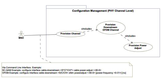
Figure 11 - Downstream RF Channel Configuration Use Case
