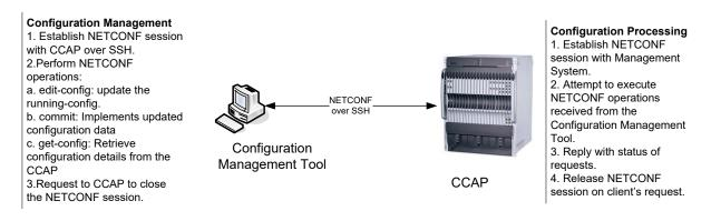
Figure 22 - CCAP NETCONF-Based Configuration Use Case
