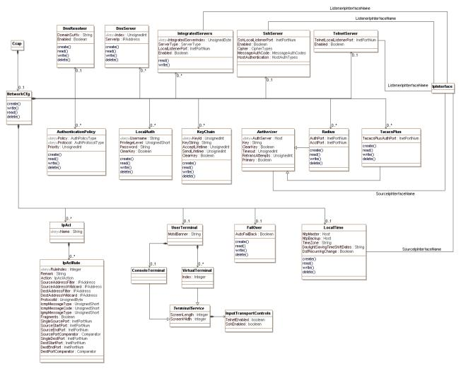
Figure 38 - CCAP Network Configuration Information Model
