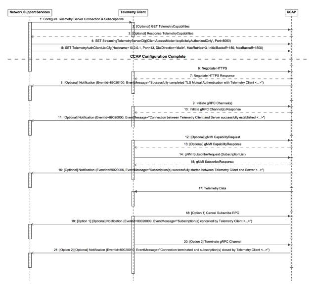
Figure 122 - Dial In Streaming Telemetry Sequence Diagram
