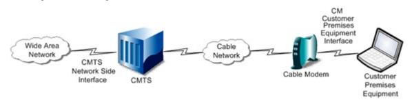
Figure 4 - Transparent IP Traffic through the Data-Over-Cable System
