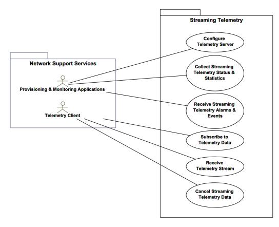
Figure 18 - Streaming Telemetry Use Cases
