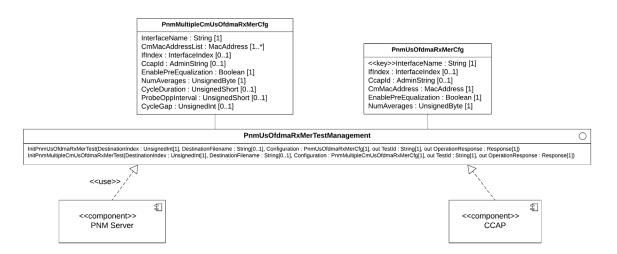
Figure 98 - PnmUsOfdmaRxMerTestManagement Component Diagram
