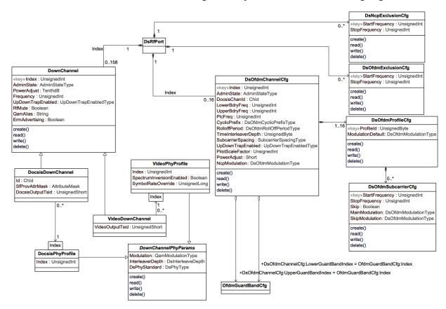
Figure 34 - Downstream DOCSIS and Video Configuration Information Model
