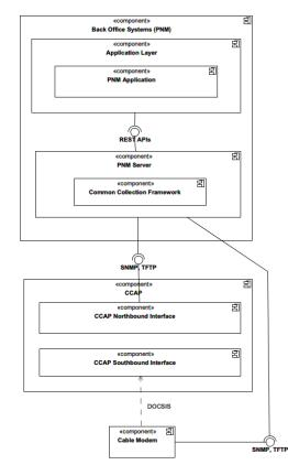
Figure 6 - Common Collection Framework for DOCSIS PNM
