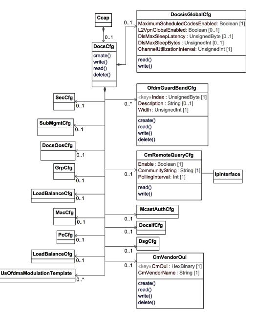
Figure 26 - DOCSIS System Configuration Information Model
