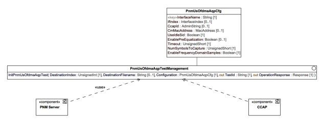
Figure 100 - PnmUsOfdmaAqpTestManagement Component Diagram
