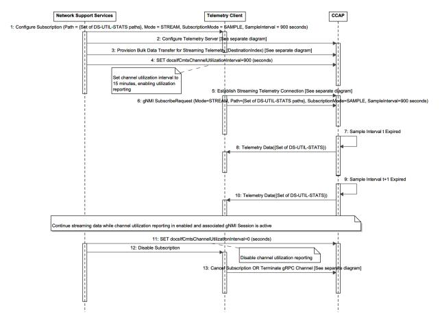
Figure 124 - gNMI Sample Streaming DS Utilization Statistics Sequence Diagram
