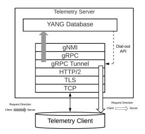
Figure 88 - Streaming Telemetry Dial-out Protocol Stack
