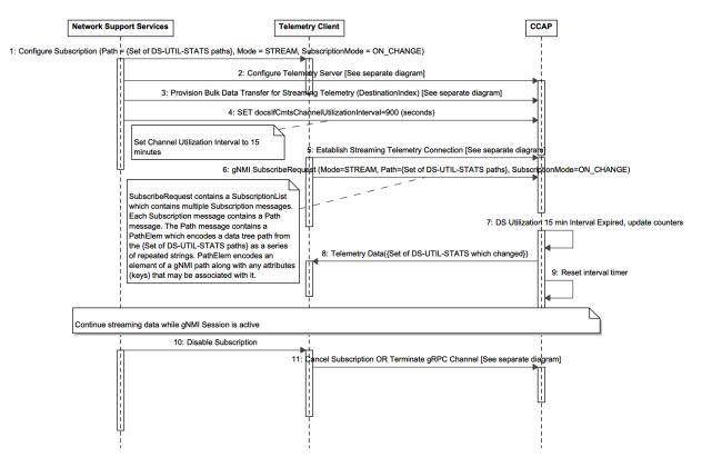
Figure 123 - gNMI On-change Streaming DS Utilization Statistics Sequence Diagram
