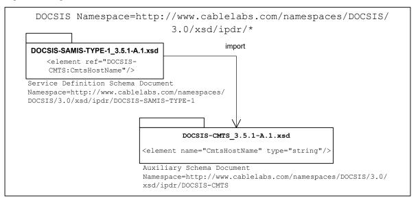
Figure 109 - Auxiliary Schema Import
