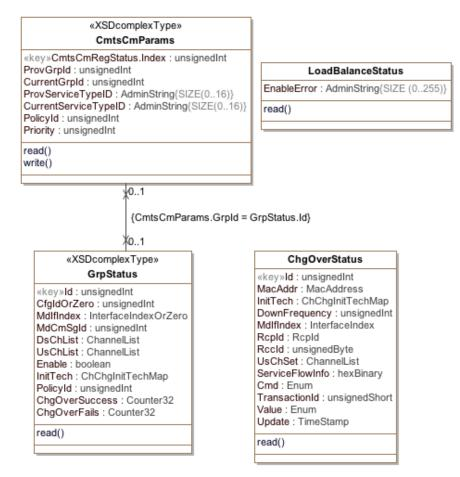
Figure 55 - DOCSIS Load Balance State Information Model
