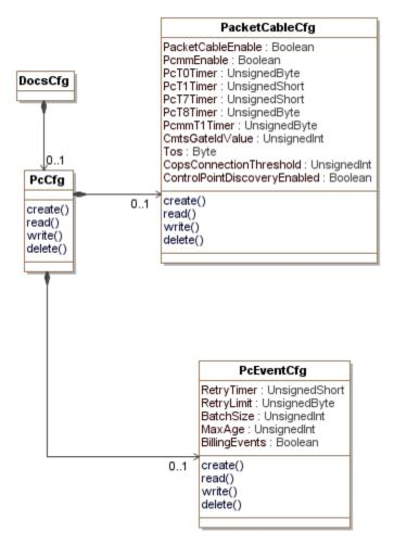
Figure 36 - PacketCable Configuration Information Model
