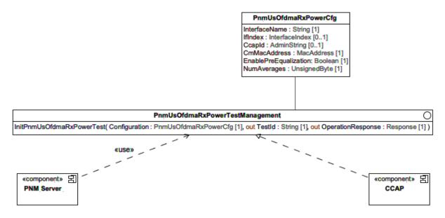
Figure 102 - CCAP PnmUsOfdmaRxPowerTestManagement Component Diagram
