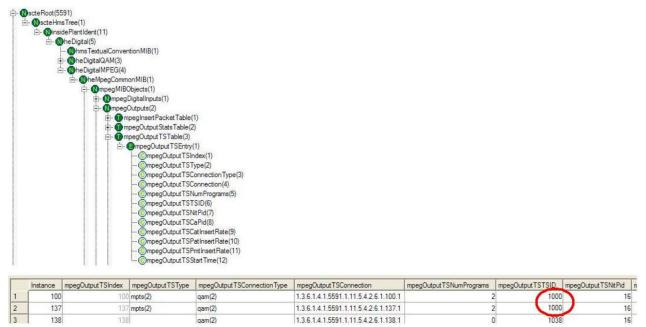
Figure 111 - Identifying a Replicated QAM by Looking at mpegOutputTSTSID
