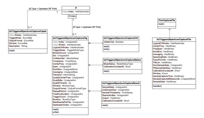
Figure 75 - Upstream Triggered Spectrum Capture Information Model
