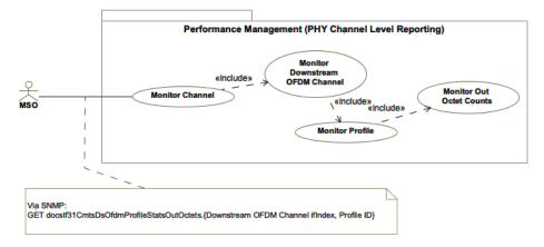
Figure 13 - Downstream Channel Performance Monitoring Use Case
