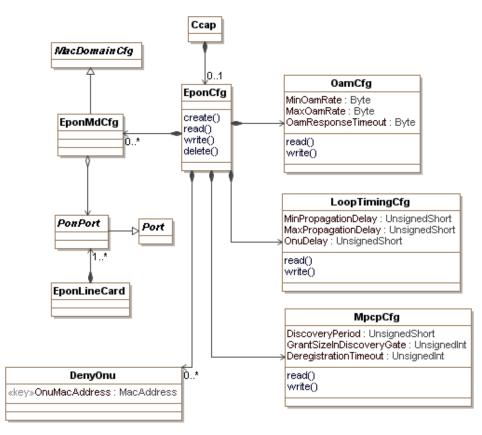
Figure 44 - EPON Configuration Information Model
