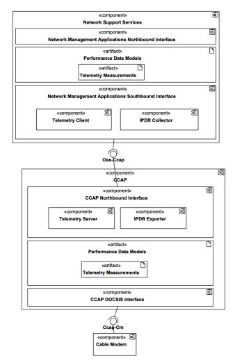
Figure 78 - CCAP Streaming Telemetry Management Architecture
