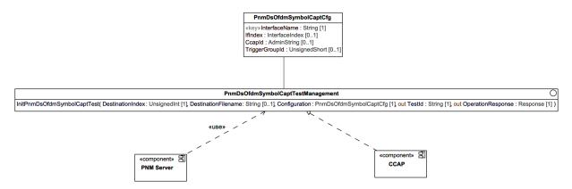
Figure 96 - PnmDsOfdmSymbolCaptTestManagement Component Diagram
