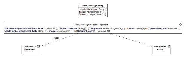
Figure 106 - PnmUsHistogramTestManagement Component Diagram
