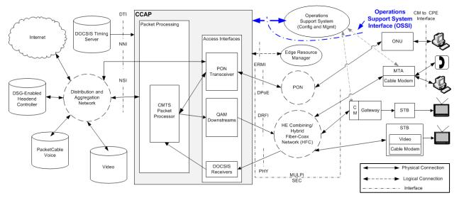
Figure 3 - CCAP Interface Reference Architecture
