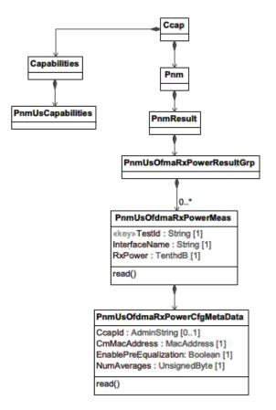
Figure 101 - CCAP PnmUsOfdmaRxPowerResultGrp Class Diagram
