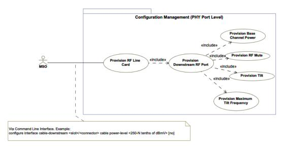
Figure 10 - Downstream RF Port Configuration Use Case
