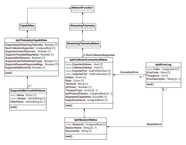
Figure 89 - IPDR Streaming Telemetry Status Information Model
