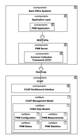
Figure 79 - DOCSIS CCF Streaming Telemetry for PNM
