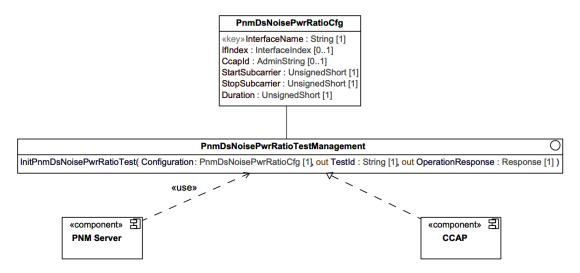
Figure 94 - PnmDsNoisePwrRatioTestManagement Component Diagram
